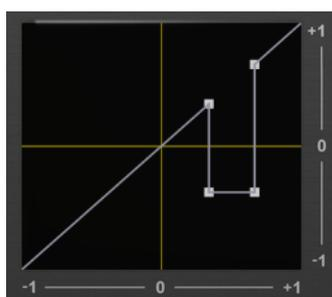
The parts of the waveform between about +0.3 and +0.6 have been mapped to a constant value
