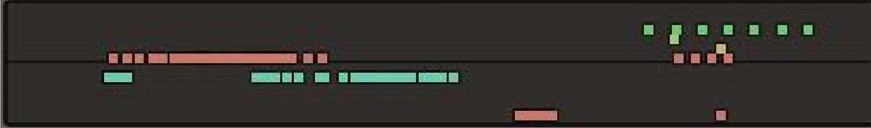
Stereo mode shows two lanes, one for each stereo channel. The top lane is the left channel, the bottom lane is the right channel. The rows are then ordered by sample slot.
