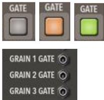
**Gate** determines whether the engine is active or not. If **Gate** is off, no grains will be created. Each grain engine has an additional CV gate input on the back. If you wish to use the CV gate, the front panel button based gate should be turned off.
