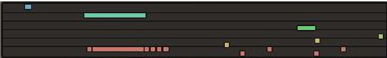
Sample mode shows six lanes, one for each sample slot. The top lane is sample slot one, the bottom lane is sample slot six. The rows are then ordered by stereo channel.
